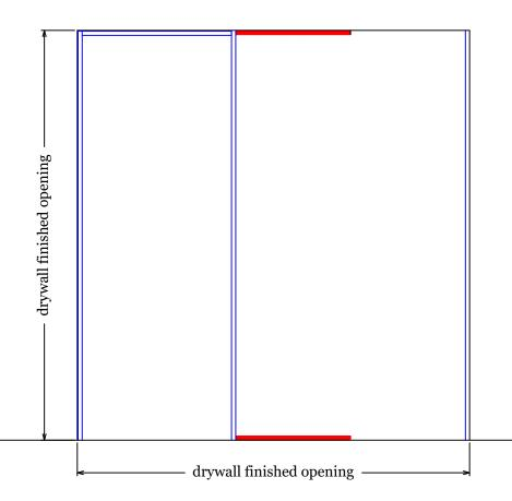
$\label{eq:step 8: Determine the length of the horizontal glass mullions and cut one side (top and bottom) and secure to the ceiling with 1-5/8" drywall screws and to the floor with the provided 1-1/4" x 3/16" TapCons - Phillips head.$
