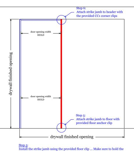
door opening width... Secure the floor clip to the strike jamb and floor
