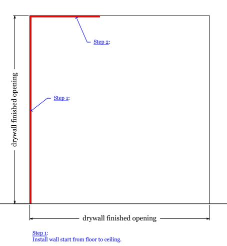
Install the wall start above the door frame header ONLY (part is cut at the factory to the exact length - do not trim)
