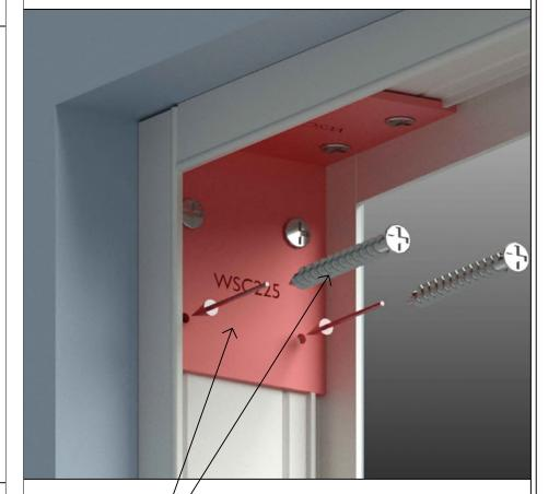
Attach wall start to drywall opening with the WSC225 clip using 1-1/4" drywall screws ....
