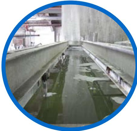
The first few steps prepare aluminum extrusions for anodizing.
