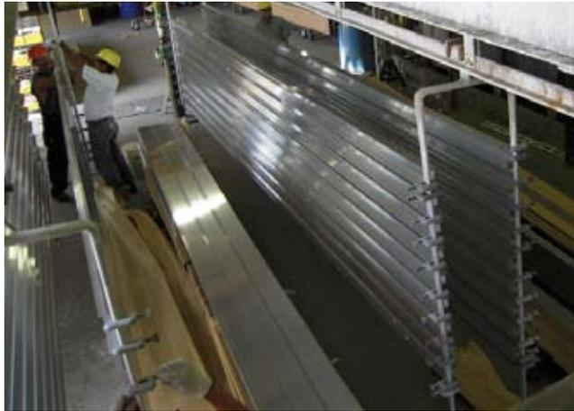
*Aluminum extrusions are securely racked prior to the cleaning tank. Our anodizing line can anodize aluminum up to 30 feet long.*
