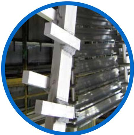
As aluminum goes through the anodizing process, the racks that hold extrusions in place corrode. Welders are available on site for this purpose!
